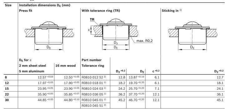
$<sup>^{</sup>f 1)}$  Made from spring hinge 1.1248 alternative 1.8159
